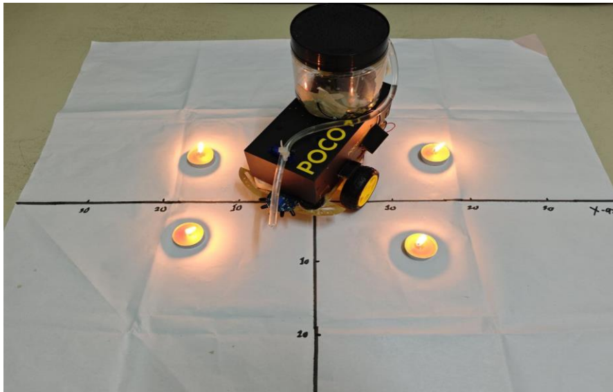
Fig. 3: Experimental test layout showing fire source positions.
